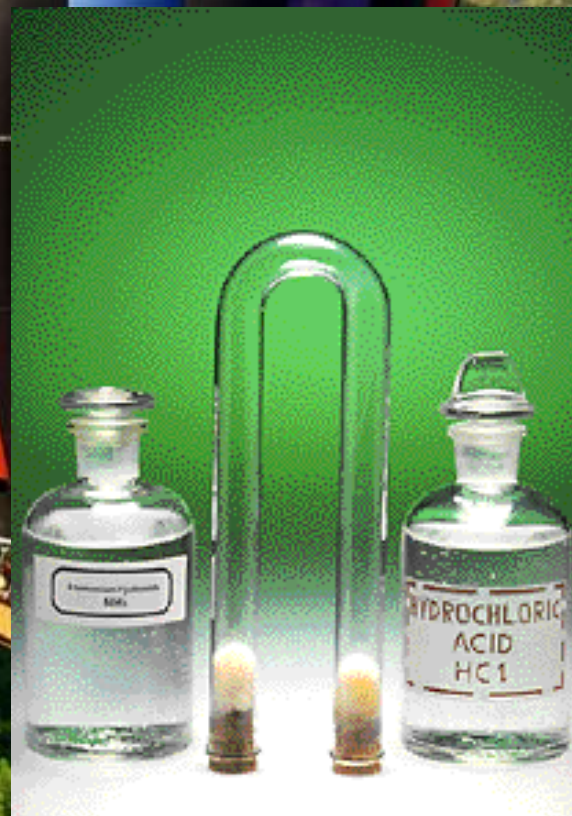
Gaseous diffusion of \text{NH}_3(\text{g}) and \text{HCl}(\text{g})
