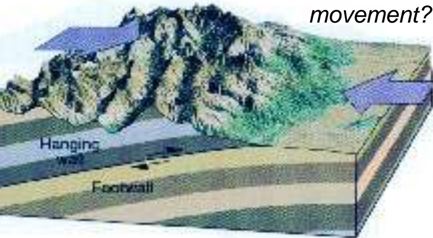
Thrust Fault - compressional
